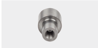
TYPE: I ROUND JET Op. pressure: up to 3000 bar Efficiency factor: 0.7 Material: Steel/sapphire Nozzles: 0.4 – 1.1 mm
