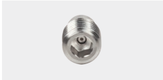
TYPE: H ROUND JET Op. pressure: up to 2500 bar Efficiency factor: 0.75 Material: Steel/sapphire Nozzles: 0.25 – 1.0 mm
