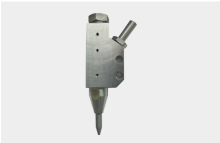
Type B 1500 Op. pressure: 1500 bar Flow rate: 25 – 40 l/min Designed to be mounted on a nozzle carrier. Applications: Concrete cutting & steelwork cutting
