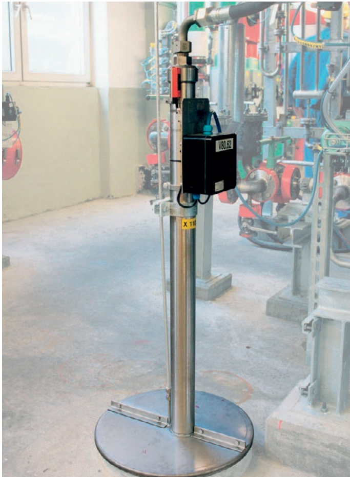
Lance system - moved hydraulically/pneumatically actuated
