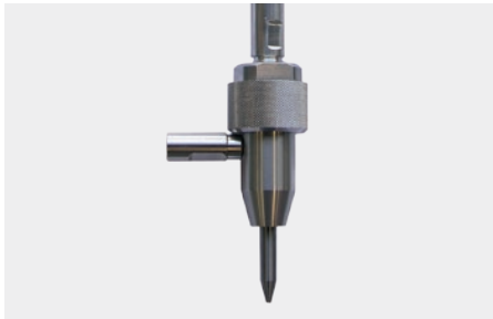
Type S 4000 (with collimation tube) Op. pressure: 4000 bar Flow rate: up to 10 l/min Applications: Especially for use with a cutting table, i.e. cutting shapes in metals, glass, plastics, ceramics etc.
