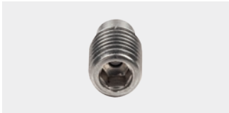
TYPE: P ROUND JET Op. pressure: up to 3000 bar Efficiency factor: 0.71 Material: Steel/sapphire Nozzles: 0.15 – 1.5 mm
