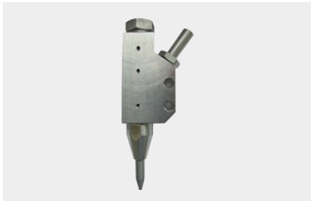
Type B 3000 Op. pressure: 3000 bar Flow rate: 10 – 25 l/min For attachment to carriage. Applications: Concrete cutting & steelwork cutting
