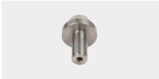
TYPE: U ROUND JET Op. pressure: up to 4000 bar Efficiency factor: 0.7 Material: Steel/sapphire Nozzles: 0.4 – 4.9 mm
