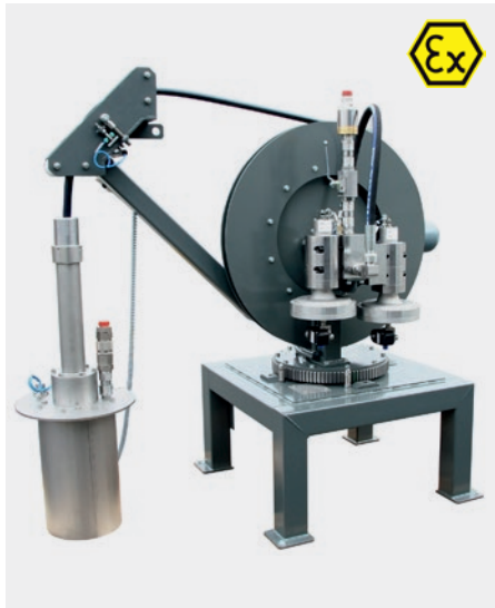
Hose reel system with jib Electrically driven hose reels. The jib is manually positioned above the opening and lowered onto the cleaning port by handheld control. The cleaning positions are freely programmable and controlled by the process plant controller.
