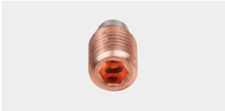
TYPE: T ROUND JET Op. pressure: up to 3500 bar Efficiency factor: 0.72 - 0.92 Material: Steel/diamond Nozzle : 0.15 – 1.00 mm
