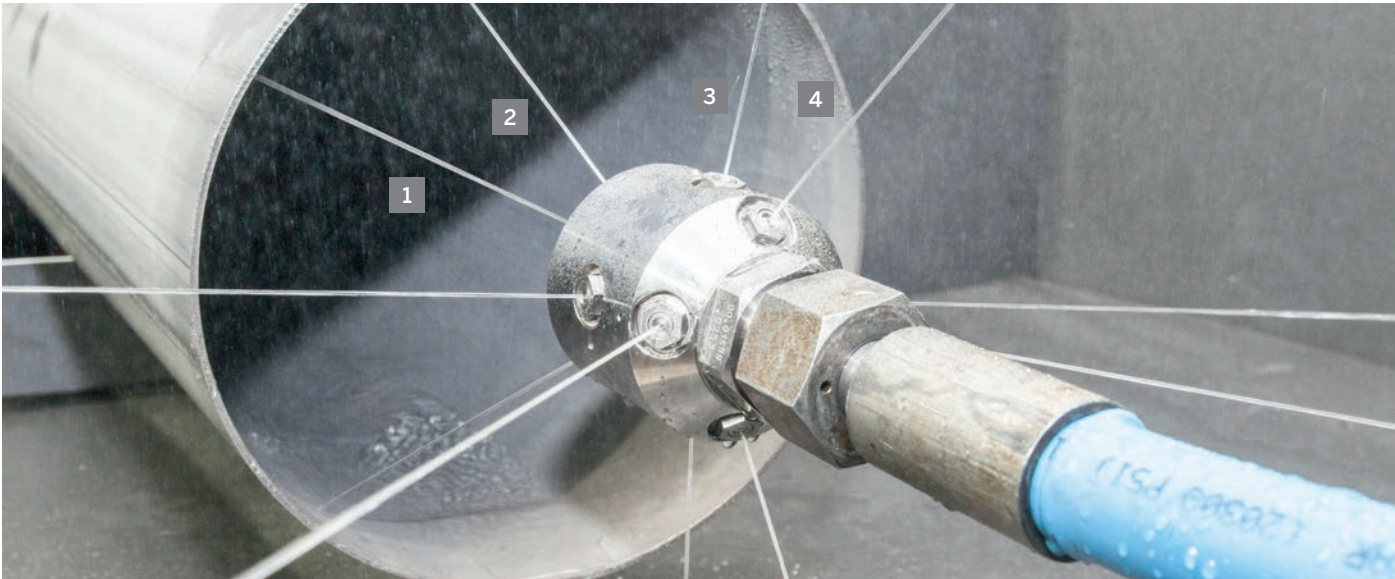
1 Axial nozzle 2 Push nozzles 3 Radial nozzles 4 Pull nozzles
